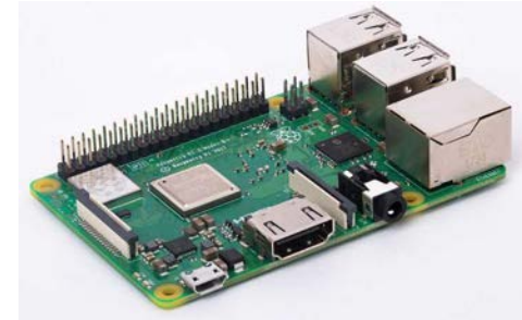
Figure 29. Single Board Computer Common in Edge Devices
